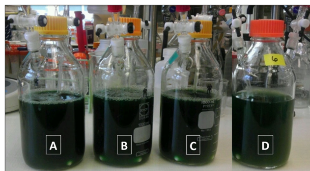
Fig. 9 Gaseous-aqueous two-phase reactors for the growth of SkIspS transformants under sealed conditions. The 500-mL headspace of the reactors was filled with 100 mL of 100 % \text{CO}_2 every 24 h. Isoprene accumulating in the headspace during photosynthesis of the cyanobacteria was quantified every 24 h, prior to refilling of the reactor with \text{CO}_2 . The cultures shown were grown for 96 h at pH 10 without added salinity (a), and with 100 mM NaCl (b), 200 mM NaCl (c), or with 600 mM NaCl (d)
